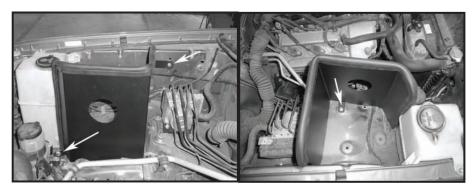
Step 11 Install the heat shield into the truck as shown with the supplied hardware.
