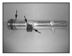
Step 10 Install the mass air flow sensor on the intake tube and secure with the supplied screws.
