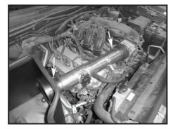
Step 13 Install the end of the intake tube into the flex coupler on the throttle body. Install the velocity adapter in the heat shield and once in place, slide the coupler from the long side of the intake onto the velocity adapter. Once the tube is in the location as shown , tighten all the clamps.
